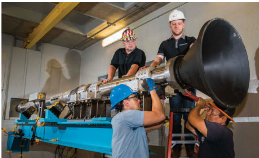
Sandia tests ensure avionics can withstand shock from stage separation in flight. (Photo: R. Montoya)
